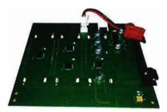
4. The M15224A001-8999 LCD Main Display is ready to be installed on the A-side of the Modular head. If being installed on the B-side, please locate the JP1 connector on the LCD Main Display and remove the jumper from JP1. Note: If JP1 jumper is placed in the "B" position, a Master Reset will be initiated once power is recycled.
