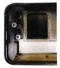
2. Install the Clear Dial Glass Insert and the new gasket onto the bezel.
