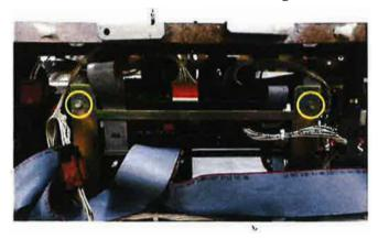
3. Disconnect the cables from the P201, P205 and P203 connectors on the SID Pump Controller board. Disconnect the Display Ribbon cable from the P204 connector and remove the cable from the Modular head to be discarded.
