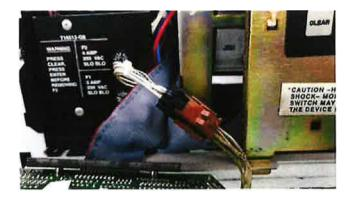
3. Disconnect the P801 Display Data cable from the SID Main Display.
