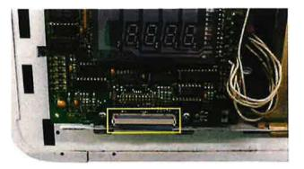
4. Remove the SID Main Display from the Modular head. Remove the mounting bracket from the bottom of the SID Main Display.
