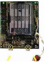
Install the bracket onto the M15224A001-8999 LCD Main Display and set aside for now.
