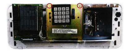
2. Remove the bracket from the Modular Card cage.
