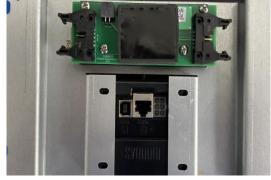
Attach the SC00002 cable between J1 on the converter board and the FIM-20.
