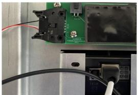
Attach the FC00004 cable between J50 on the converter board and P2 on the printer.
