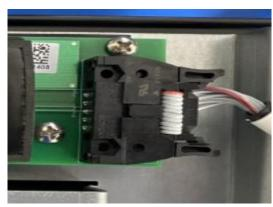
Attach the SC00013 cable between J2 on the converter board and J2 of the Easy Pump Power Supply.
