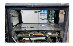
19. Mount the Power Supply Board (SC00004) onto Power Supply Bracket (SC00005) using (4) screws (6-32x3/8).
